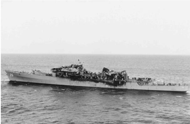
LO USS BELKNAP, COMPLETAMENTE DEVASTATO DALL'INCENDIO SCOPPIATO DOPO LA COLLISIONE CON LA USS JOHN F. KENNEDY
