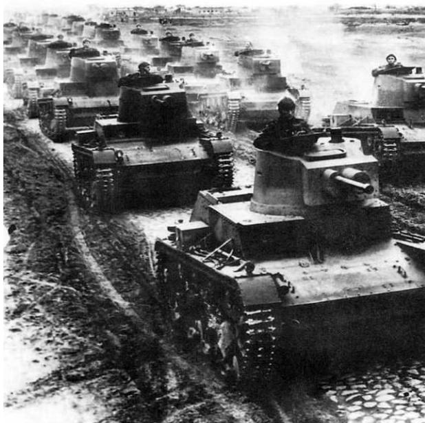
CARRO ARMATO 7TP POLACCO CON CANNONE DA 37 MM
